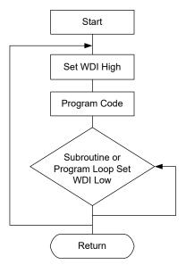
Figure 4. Watchdog Flow Diagram
