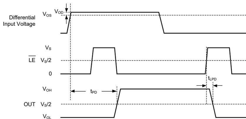
Figure 1. Timing Diagram with Latch Enable Input
